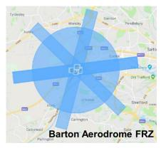
The 'standard' FRZ is a 2.5nm (4.6km) diameter circle around the centre of the airfield, with the addition of the 'stubs' extending to 5km and 1km wide in line with each runway.
